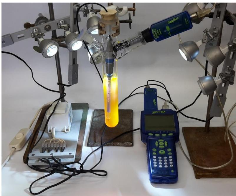
Figure 2. Pyrex irradiation chamber with two outlets for the simultaneous determination of pH, electric conductivity and temperature (in solution, central outlet) and carbon dioxide measurements in the gas phase (right outlet) and registration by means of a PASCO Xplorer GLX Graphing Data Logger.
