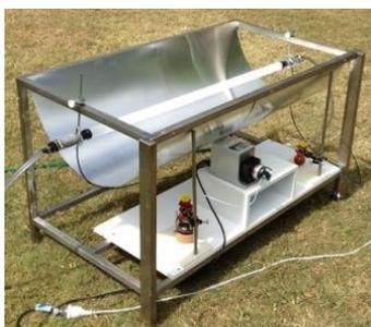
**Figure 2.** Concentrating solar trough continuous flow photoreactor.
