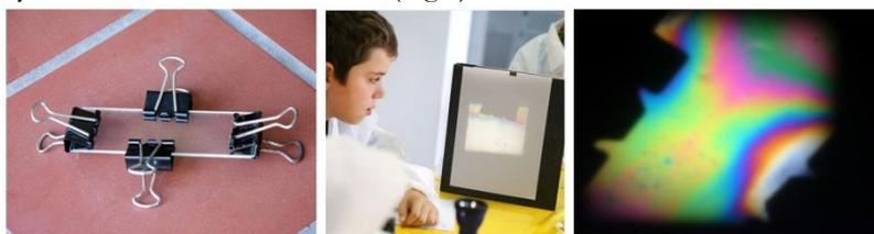
**Figure 5.** MBBA sandwich (left) and passing light at crossed polarizing filters (middle and right)
